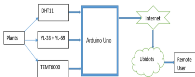
Fig 4. Block diagram of plant health monitoring system [27]
