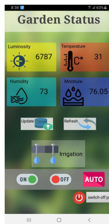
Fig 13. Smart IOT Garden App (Automatic Irrigation)
